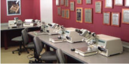
**WEST-BOND's** 7300C Series pick up and place chips for manual die attachment by mechanical scrub, eutectic method. All operation is controlled by West-Bond's unique three-axis micromanipulator under microprocessor control. The work piece is held on a heated work holder, where chips are also arrayed for pick up.
